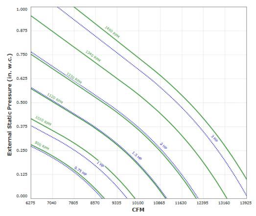
Max Sizeable RPM = 1450 RPM. Curve shown extended beyond this point for reference only.
